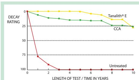
The graph shows that small samples of TANALITH® E pressure treated timber are providing outstanding performance in an aggressive field test site, even after 10 years exposure. This demonstrates that professionally treated commercial sized timbers can achieve a desired service life of 15 years or more in ground contact.
